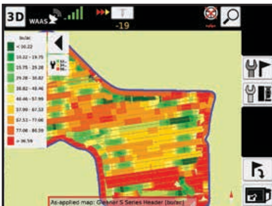
Gleaner Tyton terminal screen showing FieldStar Live real-time yield mapping.
